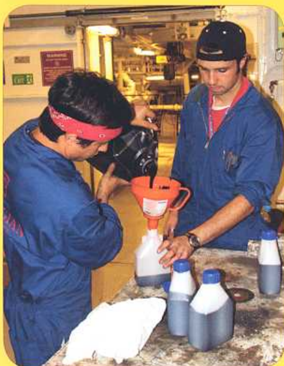
The ship's Second Engineer Joe Clark (left) working together with Oiler Curtis Tobey to collect samples for oil analysis in the engine room of the PRIDE OF AMERICA. (Photo courtesy of SIU's Mike Hickey/Jordan Biscardo).
