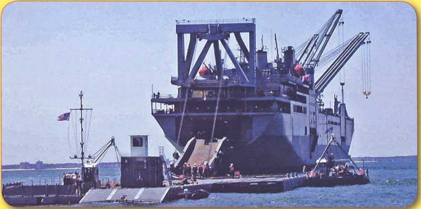
The STOCKHAM unloading Navy vehicles utilizing its capacity as a Roll-On/Roll-Off vessel.
